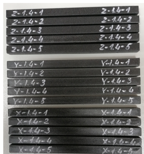
Figure 5. Examples of identified specimens before the flexural tests.
