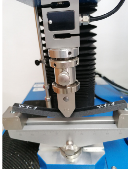
Figure 6. Specimen subjected to bending.
