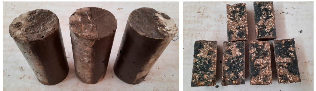
Figure 6. Samples configuration and failure patterns of composite normal strength concrete substrate and SFRGPC repair material.
