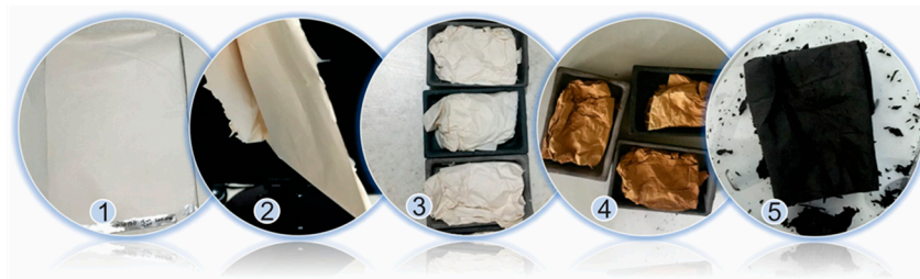
Figure 3. Photos of fibers after thermal stabilization processes and carbonization: (1) fibers from 30/70 lignin/PAN on the substrate; (2,3) the type of fibers removed from the substrate; (4) fibers after the thermal stabilization process; (5) fibers after the carbonization process.
