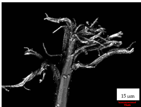
Figure 2. Confocal microscope image, fibrillation of cotton fiber ends.
