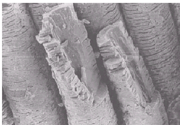
Figure 3. Consequence of oxidative degradation of PP fibers.
