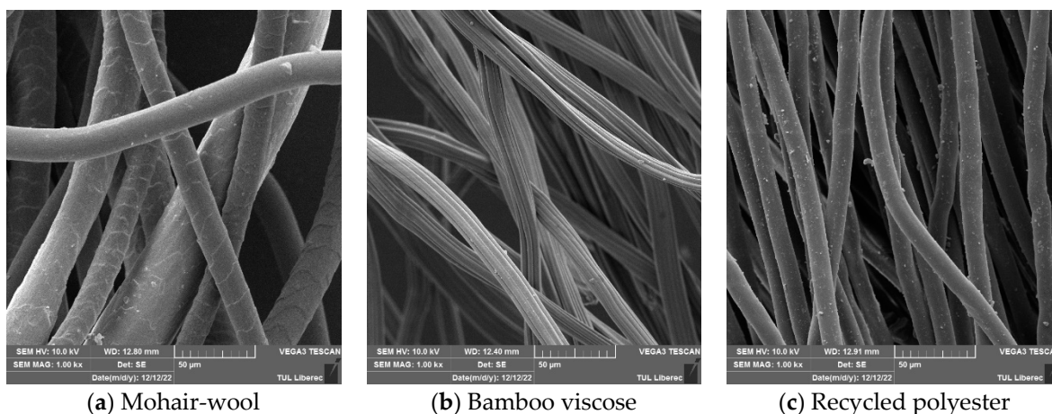
Figure 8. SEM images illustrating the physical structure of the fibres in the 3 main yarns used in this study. With (a) fibres in a yarn referenced as MW (mohair-wool), (b) yarn BV (bamboo viscose), and (c) yarn PETR (recycled polyester). The SEM magnification is 1000x and the images show a clear difference in the surface characteristics of the fibre types.
