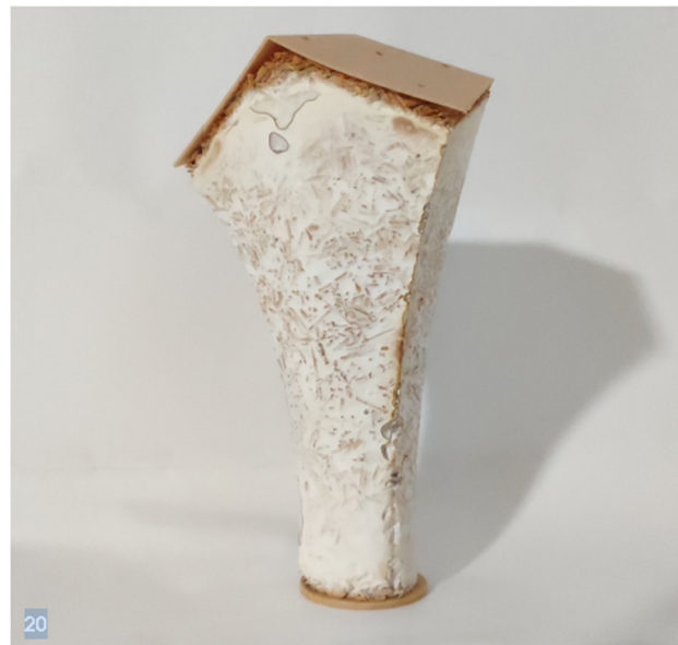
Figure 2. Building element from ganoderma lucidum mycelium cultivated in a hemp fiber substrate. One of the three types of building elements with different geometry produced in the context of a diploma thesis in the Department of Architectural Engineering.
