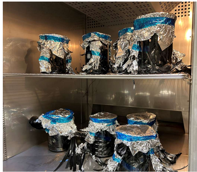
Figure 1. Aging of fiber samples inside an oven.
