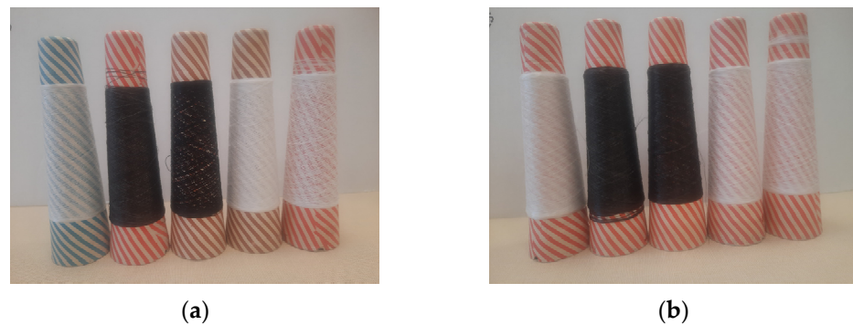
Figure 2. Prepared pure PLA and color PLA fibers. (a) PLA I6100D and (b) PLA L175.
