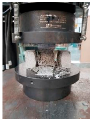
Figure 4. Compressive strength measurements.
