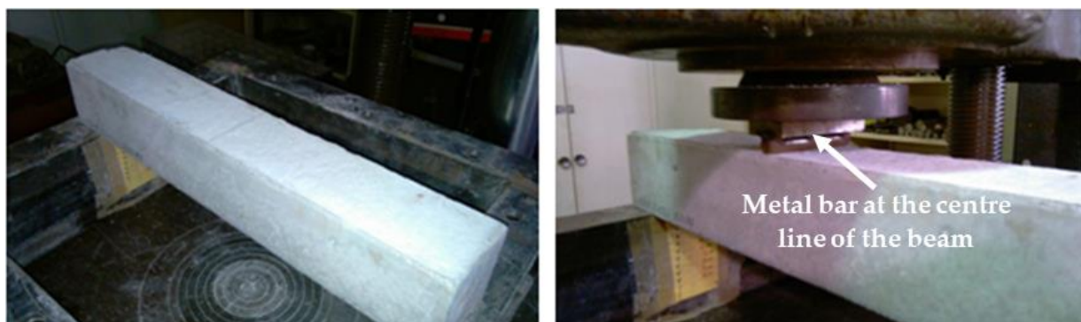
Figure 2. Static load test setup.
