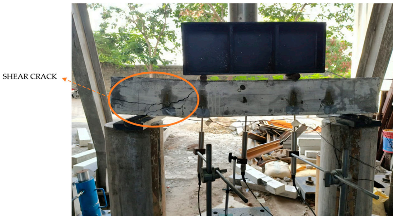
Figure 11. Crack pattern developed in TRC beam.
