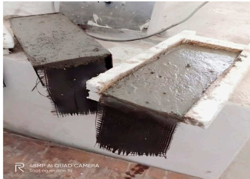
Figure 4. Pull out test specimen.
