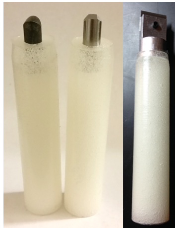
Figure 1. Projectiles used for transverse impact into yarn material. From left to right can be seen the 0.30-cal round, 0.30-cal FSP and razor blade projectiles [12].
