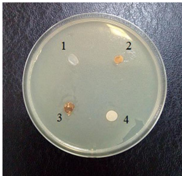
Figure 8. Evaluation of the antimicrobial activity of films with respect to Escherichia coli : 1 composite film (95% cellulose + 5% betulin), 2 filter paper, saturated with mycelium extract of Laetiporus sulphureus strain, 3 bacterial cellulose film, saturated with mycelium extract of L. sulphureus strain, 4 filter paper, wetted pyrogen-free water (control).
