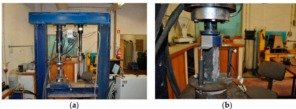
Figure 3. Uniaxial compressive strength (UCS) test set-up: (a) general view; (b) test in progress.
