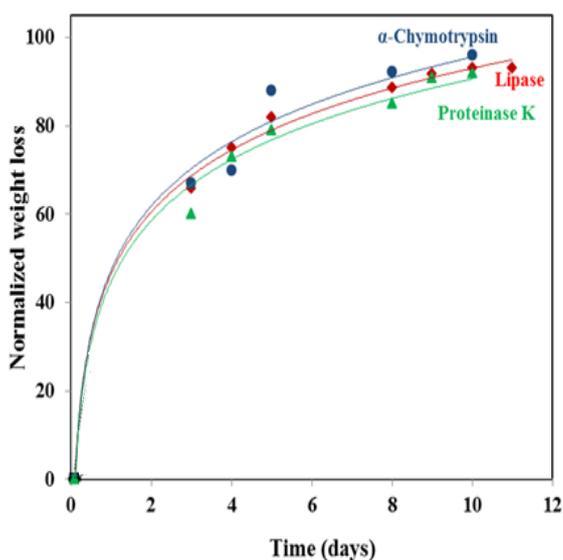
**Figure S5.** Plots of weight loss versus exposure time for 1L6 scaffolds exposed to proteinase K (green symbols)  $\alpha$ -chymotrypsin (blue symbols) and lipase (red symbols) media. Reproduced with permission from [2], copyright 2015 Elsevier.
