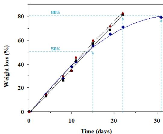
**Figure S3.** Plots of weight loss versus exposure time for 1L6 films exposed to proteinase K (black symbol),  $\alpha$ -chymotrypsin (garnet symbol) and lipase (blue symbol) media. Reproduced with permission from [2], copyright 2015 Elsevier.
