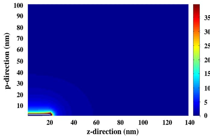
**Figure S7.** Calculated modulus of the electric field for a potential of 30 kV.
