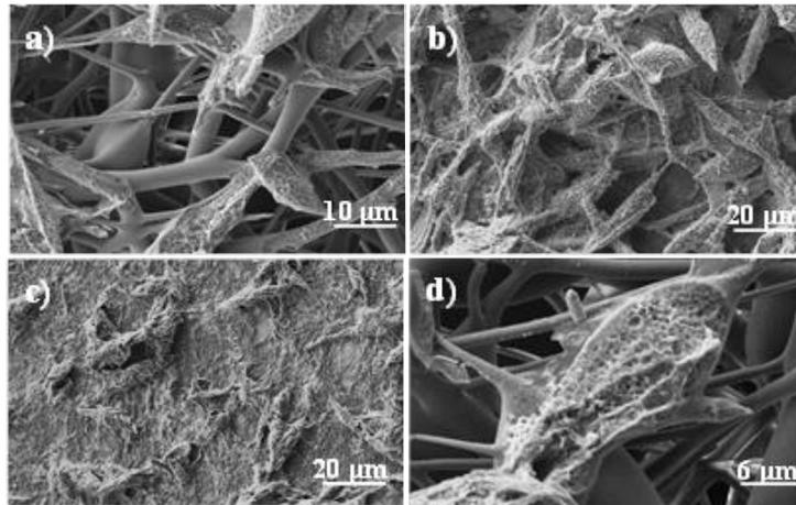
**Figure S6.** SEM micrographs of 1L6 scaffolds after exposure to an  $\alpha$ -chymotrypsin medium at 37 °C for 3 (a,d), 6 (b) and 8 (c) days. Reproduced with permission from [2], copyright 2015 Elsevier.
