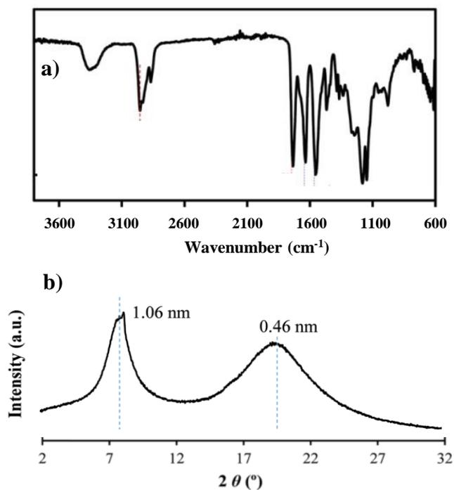
**Figure S2.** FTIR spectrum (a) and X-ray diffraction profile (b) of poly(ester urea) 1L6.
