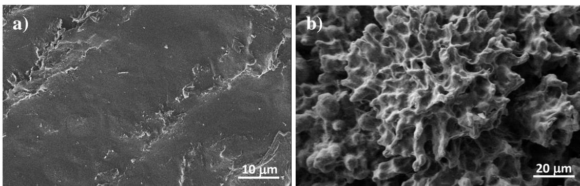
**Figure S4.** Scanning electron micrographs of 1L6 films after 19 days of exposure to PBS (a) and  $\alpha$ -chymotrypsin (b) media at 37 °C. Reproduced with permission from [2], copyright 2015 Elsevier.
