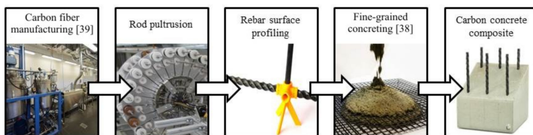
Figure 1. Process chain for the manufacturing of carbon concrete composites (reproduced with permission from [38,39]).
