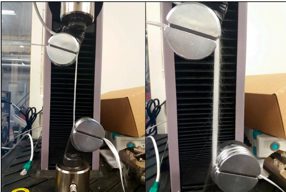
**Figure 1.** Tensile tests of R-glass fiber bundles: (left) the test is running; (right) the glass fiber bundle has failed.
