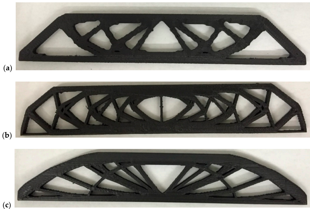
Figure 7. Printed optimized MBB beams: (a) CFAO optimized beam from Figure 4, (b) optimized for fixed horizontal print direction ( \theta_e = 0 ) (Adapted from Reference [45]), and (c) optimized for fixed vertical print direction ( \theta_e = 90^\circ ) (Adapted from Reference [45]).
