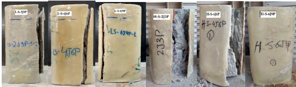
Figure 9. Failure modes of low- and high-strength square columns.
