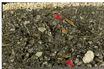
Figure 6. Voids between the fiber and the matrix (cross section).
