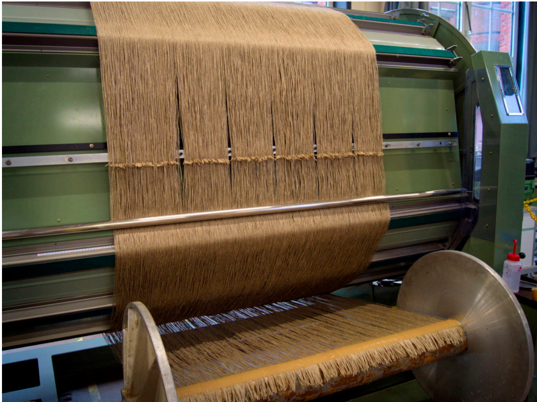
Figure 2. Stuffer warp yarns beam on sample warping machine.
