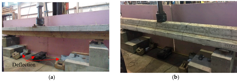
Figure 7. Test arrangement: (a) the non-inverted T-beam for positive curvature; (b) the inverted T-beam for negative curvature.
