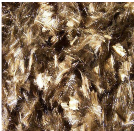
Figure 1. Basalt fiber appearance obtained by optical microscopy.
