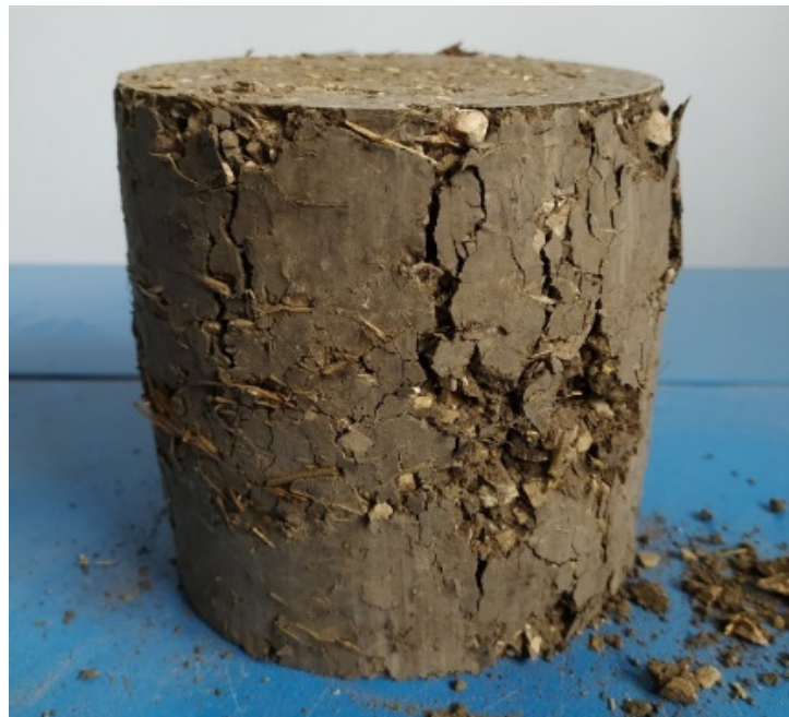
Figure 7. Failure of the specimens of compression test.
