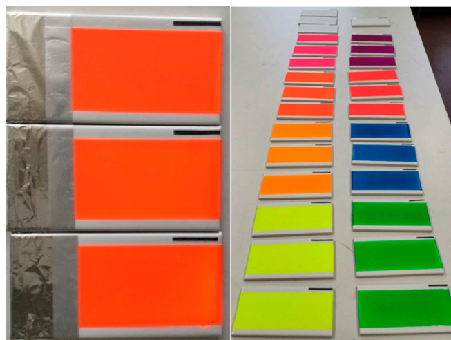
Figure 3. Sample preparation of the Kremer Fluorescent Orange (left) and all nine pigments (right) in Golden Acrylic Matte Medium prepared on white ceramic tiles.
