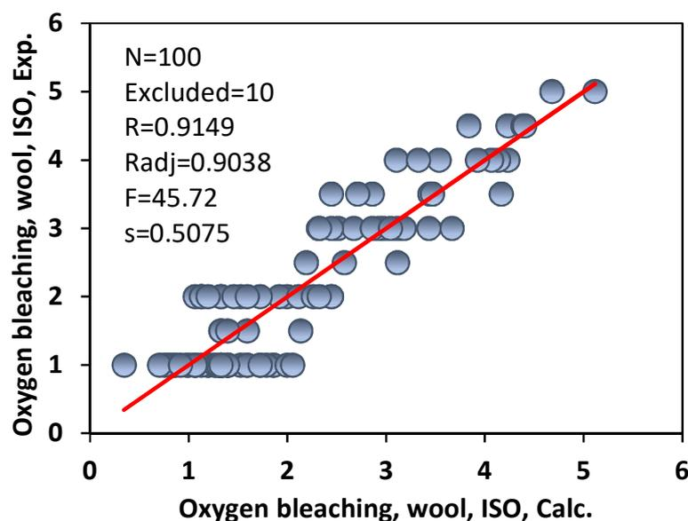
**Figure 2.** Correlation between calculated and experimental values of oxygen bleaching sensitivity of commercial azo acid dyes on wool fibres.
