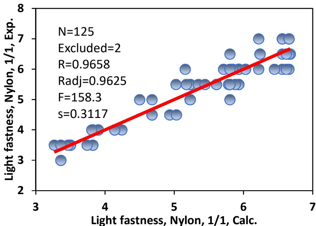
**Figure 4.** Correlation between calculated and experimental values of light fastness of dyeings on polyamide fibres.
