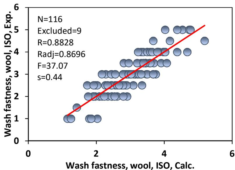
Figure 3. Correlation between calculated and experimental values of wash fastness of commercial azo acid dyes on wool fibres.
