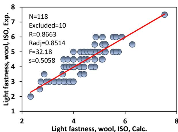
**Figure 1.** Correlation between calculated and experimental values of light fastness of commercial azo acid dyes on wool.
