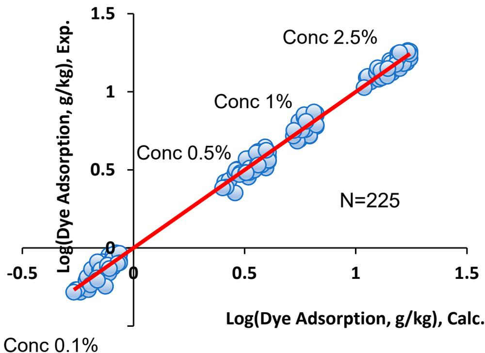
**Figure 5.** Correlation between calculated and experimental values of dye adsorption on cotton.
