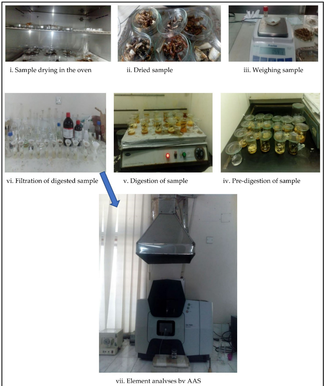
Figure 2. Main steps of heavy-metal analyses using AAS.
