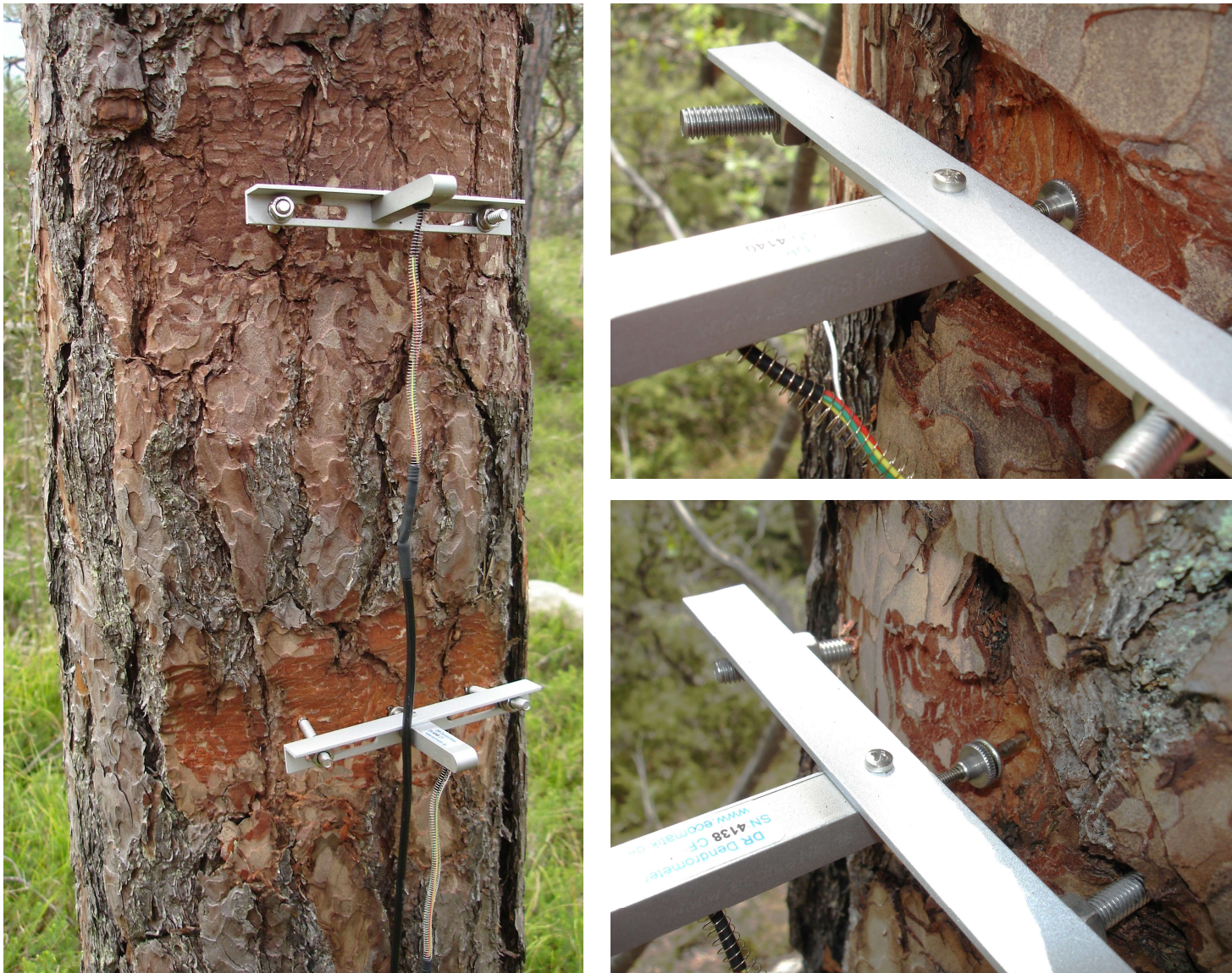
Figure S1. Overview (left) and close-up (right) of point dendrometers mounted on the bark (top; dead outer bark layers were removed) and on the xylem (bottom; sensor positioned on a screw, which was inserted c. 2–3 cm into the sapwood) of a sample tree ( Pinus sylvestris L.).
