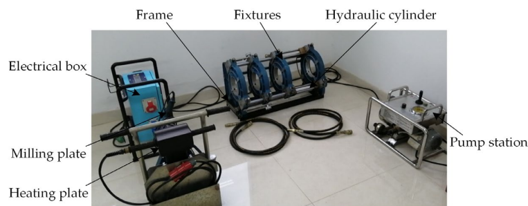
Figure 16. PE pipeline hot-melt welding machine.
