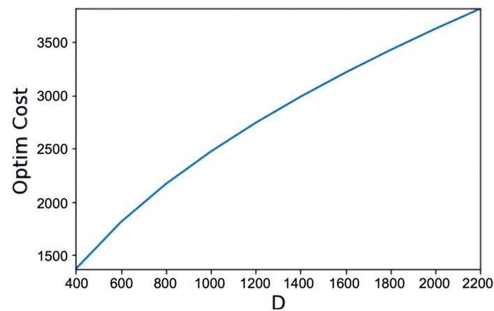
Figure 5. Optimal total cost curve varying with the demand rate of minor item.
