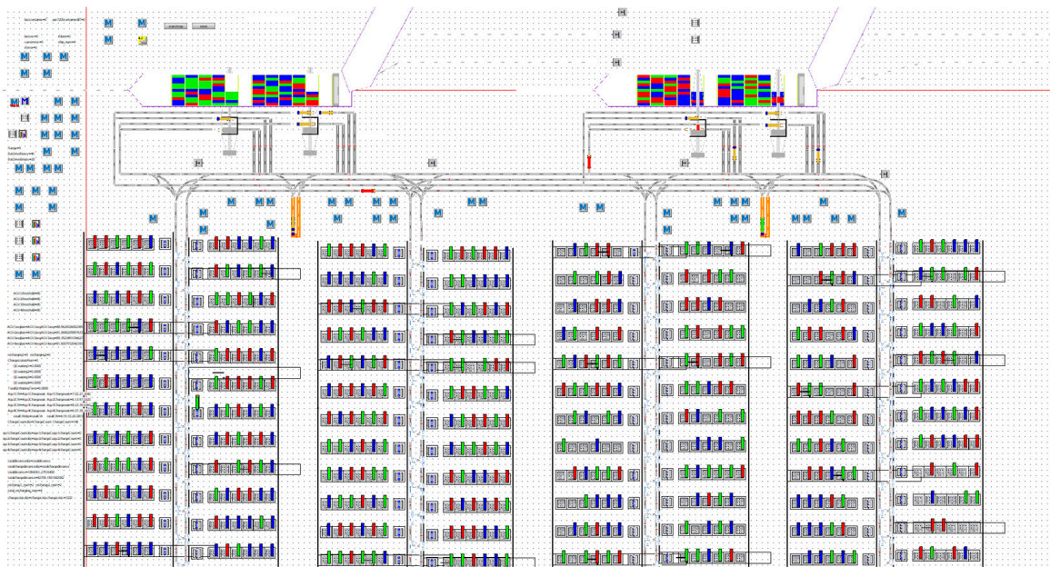
Figure 8. Schematic diagram of U-shaped automated container terminal simulation model.
