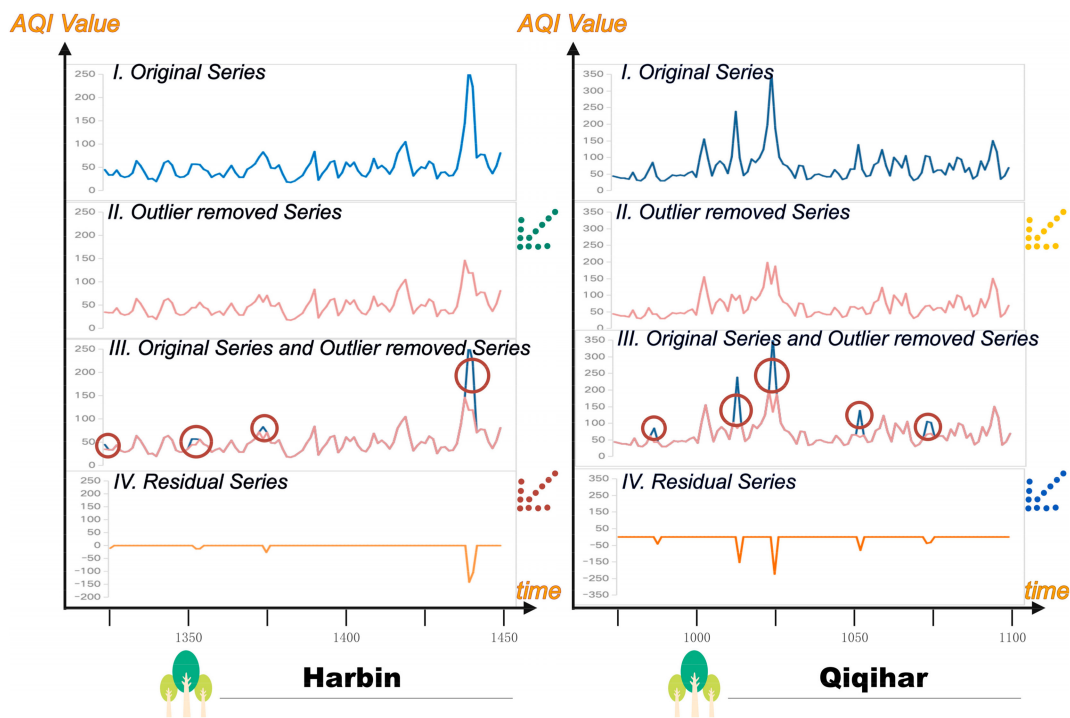
Figure 3. The data processing principle of Hampel filtering.
