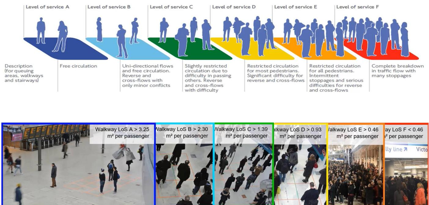
**Figure 10.** LOS used in LEGION to represent the congestion in different mobility spaces [3,6].
