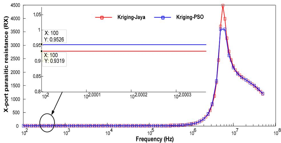
Figure 11. HSPICE simulation of Rx of CMOS OTA based CCII+: Kriging-PSO vs. Kriging-JAYA ( $I_{bias2} = 10 \mu A$ ).
