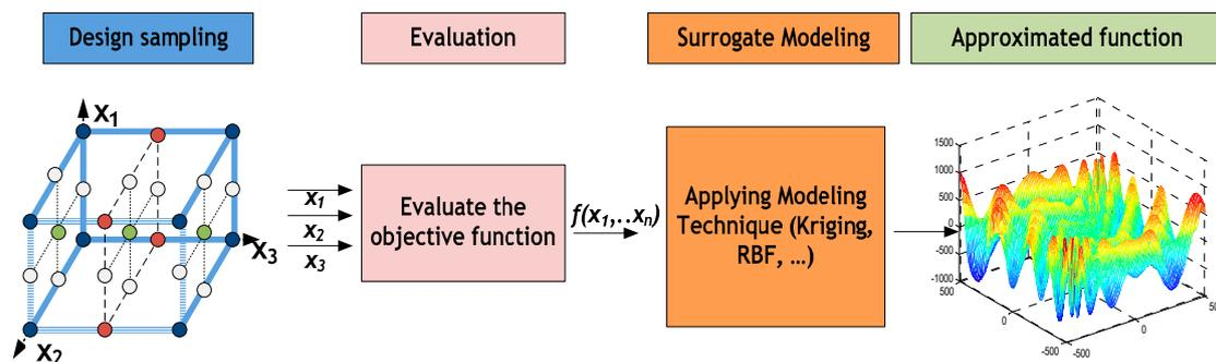
Figure 1. Steps to construct surrogate models.
