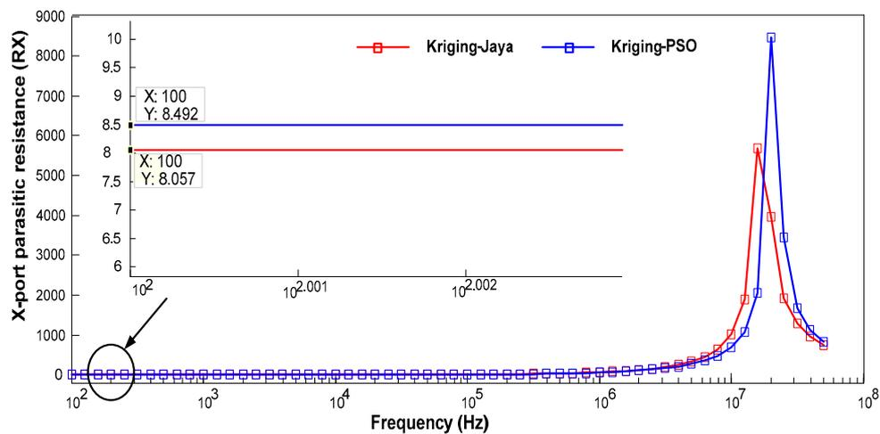
Figure 8. HSPICE simulation of Rx of the differential-based class AB CMOS CCII: Kriging-PSO vs. Kriging-Jaya ( $I_{bias} = 10 \mu A$ ).
