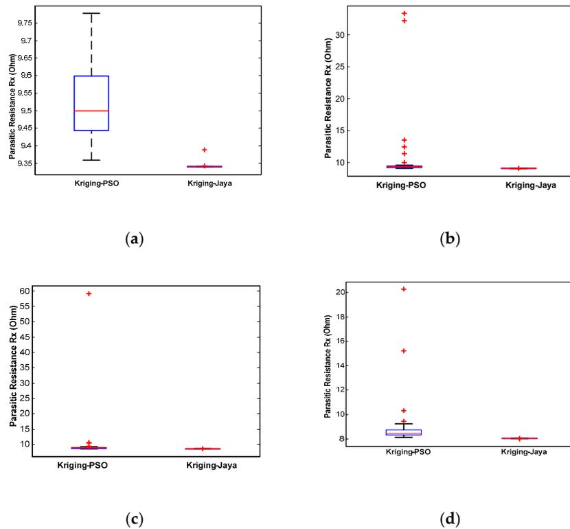
**Figure 9.** Boxplot of the 50 execution results for Kriging-PSO and Kriging-Jaya regarding Rx performances of the differential-based class AB CMOS CCII.  $I_{bias} =$  (a) 100 nA, (b) 250 nA, (c) 1  $\mu$ A, (d) 10  $\mu$ A.
