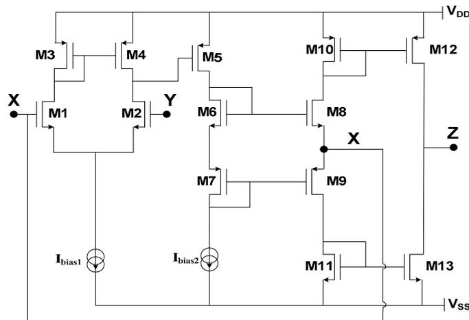
Figure 10. A CMOS OTA based CCII+.
