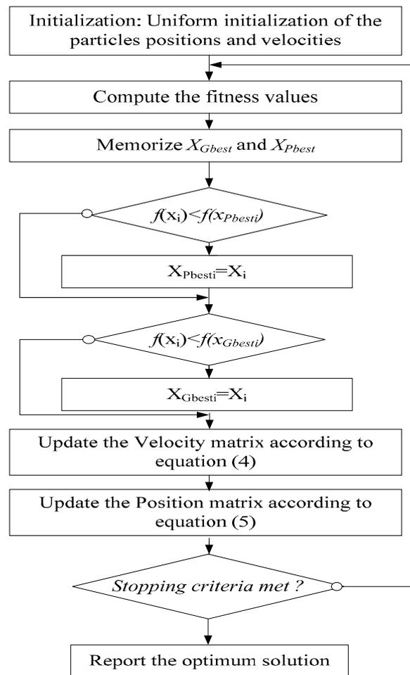
Figure 2. The PSO algorithm flowchart.
