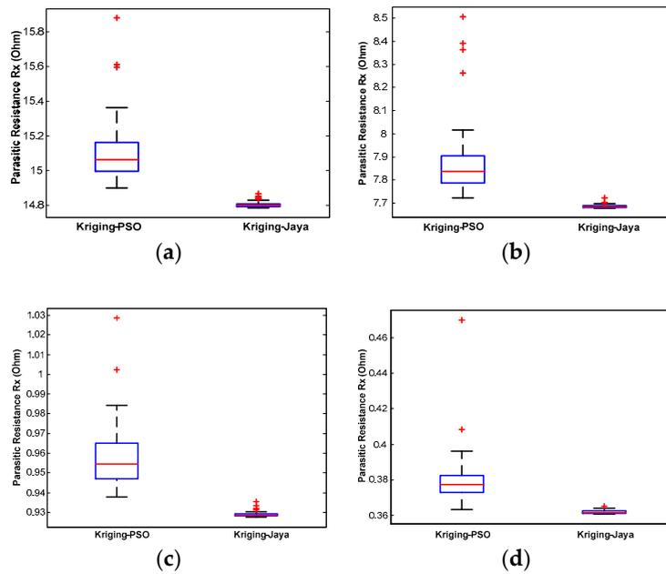
**Figure 12.** Boxplot of the 50 execution results for Kriging-PSO and Kriging-Jaya regarding Rx performances of CMOS OTA based CCII+.  $I_{bias2} =$  (a) 500 nA, (b) 1  $\mu$ A, (c) 10  $\mu$ A, (d) 30  $\mu$ A.
