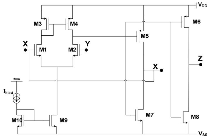
Figure 7. Differential-based class AB CMOS CCII.
