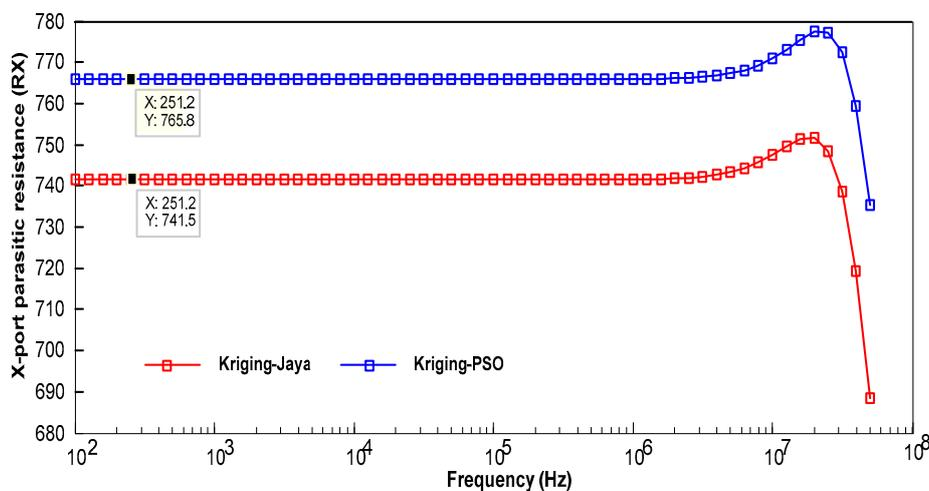
**Figure 5.** HSPICE simulations of Rx of Class AB CMOS CCII+: Kriging-PSO vs. Kriging-Jaya ( $I_{bias} = 26 \mu A$ ).
