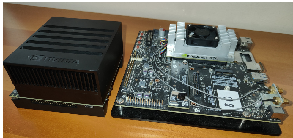
Figure 14. The embedded platforms used for testing. The Nvidia Jetson Xavier (left) and Nvidia Jetson TX2 (right).
