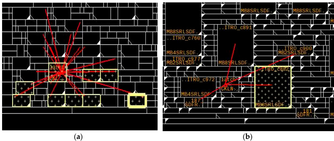
Figure 3. Example of 8-bit MBFF merging (Layout View): (a) Before the merge; (b) After the merge.
