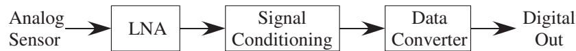
Figure 5. Block diagram of classic analog architectures to move analog signals to as high a digital SNR representation as possible. Moving digital signals to as high SNR analog representation has a similar diagram. All classic analog system design (e.g., [31]) follows This path, whether it be accoustic, ultrasound, or accelerometer sensing from a microphone to digital representation, CMOS image sensor (two-dimensional processing), or antennas for wireless processing.
