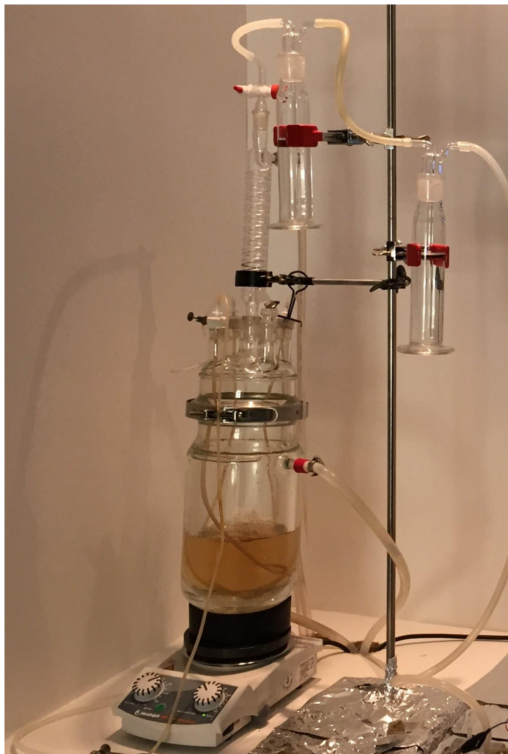
Figure S1. Glass fermenter connected to a thermostat water bath, a reflux condenser and to an exit system containing NaOH solution. Note that in order to purify H 2 from H 2 S, gas produced during fermentation process first passes through a flask containing NaOH solution (2M) and a second flask containing distilled water.
