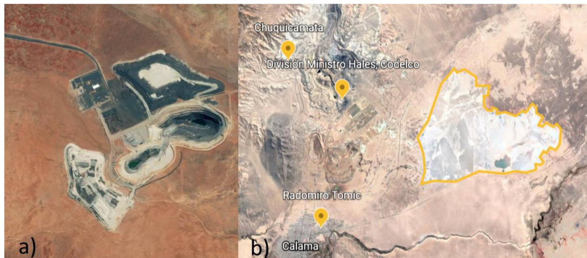
Figure A3. (a) Cairn Hill mine, Australia: No TSF was visible on satellite imagery. Dry stacking of tailings was assumed, and the mine was omitted from the dataset since only wet tailings were considered relevant for dam failures. (b) Presumably shared TSF between Chuquicamata, Radomiro Tomic and Ministro Hales mines in Chile. The measured surface area of 66.5 km 2 was split according to the relative copper output of each mine. Vice versa, in cases where multiple TSFs belonged to a single mine, their surface areas were added. The image also illustrates how TSF boundaries could not always be clearly distinguished. Areas which looked as if they had run dry (dark brown) were not included. Differences to TSF areas from 2015 reported by Werner et al. [40] were found to be small and therefore acceptable.; Images: Google, © 2022 Maxar Technologies, CNES/Ai.rbus.
