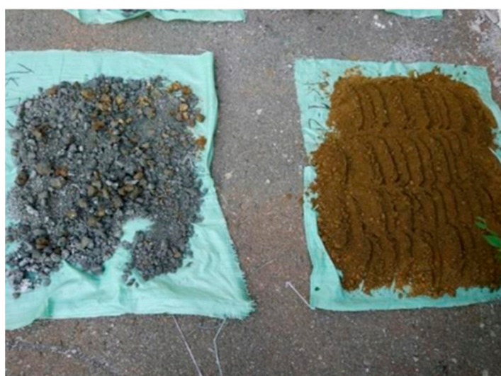
Figure S2. Identified two separate fractions with different content of non-ferrous and noble metals (old tailings of the Sibayskiy Ore-Processing Plant).
