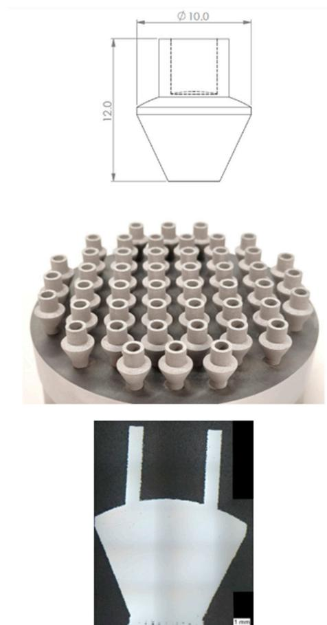
**Figure 3.** Near net shape AM electrode head (numbers in mm), AM batch production, and cross section.
