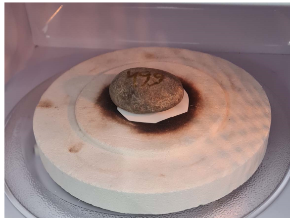
Figure 3. A sample of chert gravel after irradiation. Subjecting the sample to irradiation for 1–2.5 min did not result in crushing or any visible alteration in its shape.
