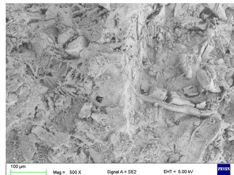
**Figure 4.** Structure of hybrid soil modifier after the tests—hydrated, dried, and hygienized R-SPA mixed with cellulose fibers from AHP and HAL (SEM).
