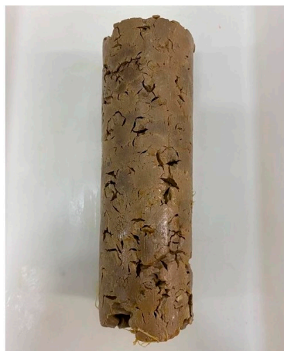
Figure 2. Aspect of the plug formed by pellets hydrated directly in water, following the methodology proposed for onshore wells.
