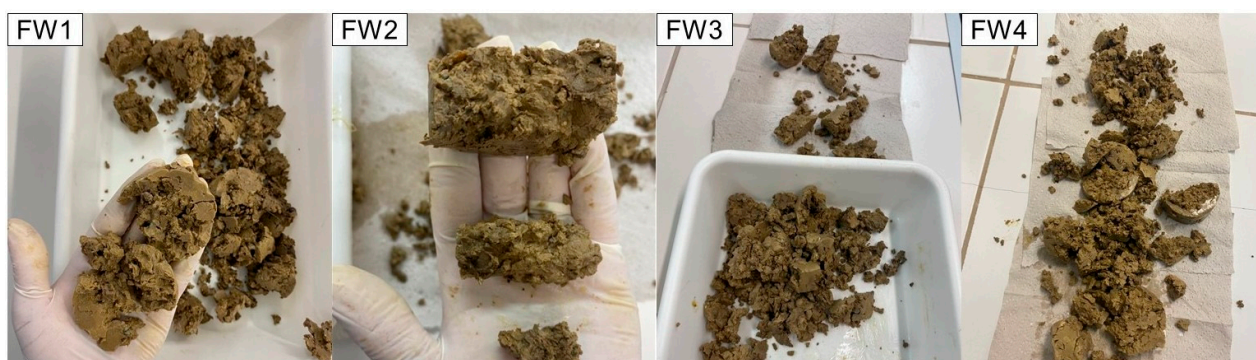
Figure 4. Offshore plugs (diesel) after contact with synthetic formation waters.
