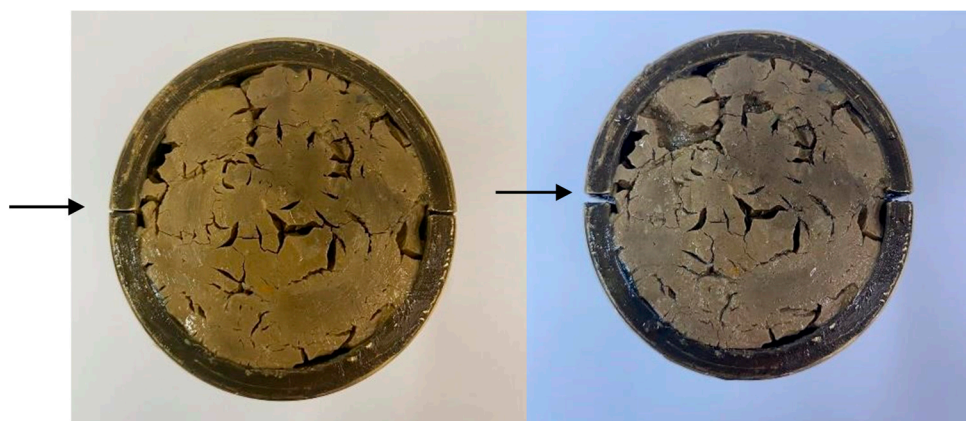
Figure 8. Opening between the plates of the metal mold due to the swelling of the plug immersed in FW3.
