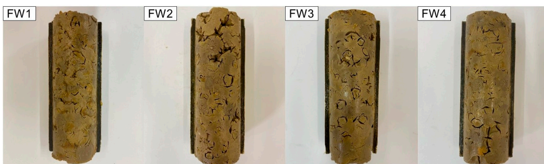
Figure 7. Appearance of onshore plugs after immersion in each formation water.
