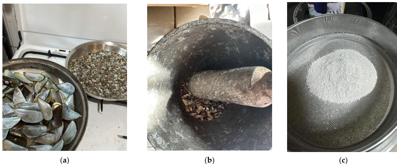
Figure 2. Experimental photos when (a) heating, (b) pulverizing, and (c) sieving the green mussel shells.
