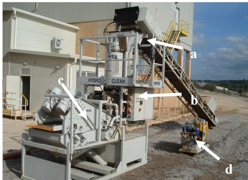
Figure 2. Pilot-scale washing installation Hydro-Clean HC 350 device: (a) Feeder, (b) washing unit, (c) de-watering screen, (d) power source [19].
