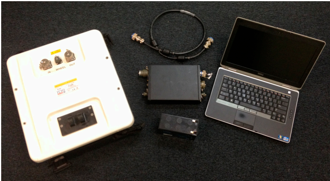
Figure 2. Commercial GPR system utilized for the coal seam sensing system. The items consist of an antenna (left), controller and cable (centre), computer (right) and 12V battery (centre bottom).
