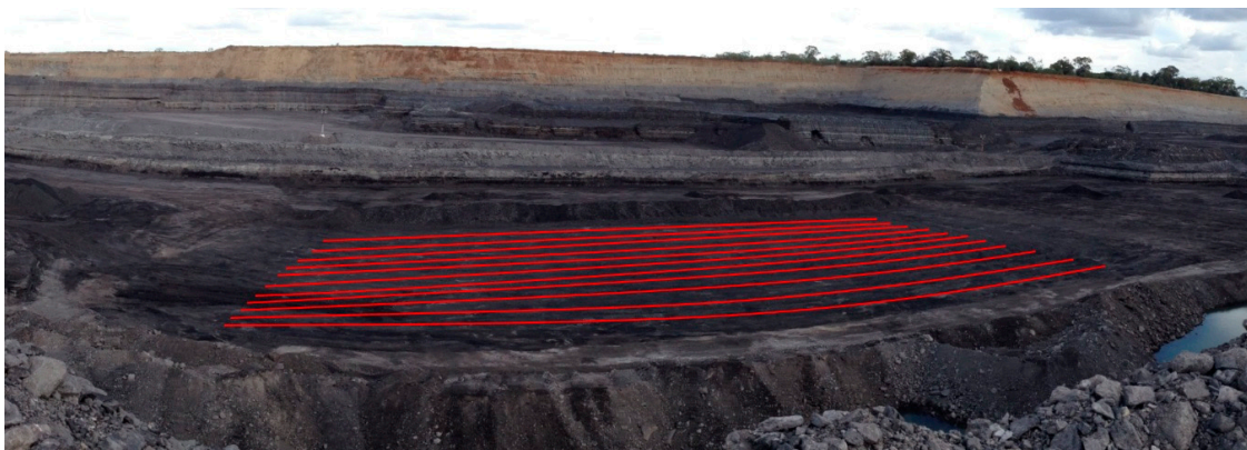
Figure 9. Area of an open cut coal mine surveyed to evaluate the sensing system. The red lines represent the path taken by the scanning system.
