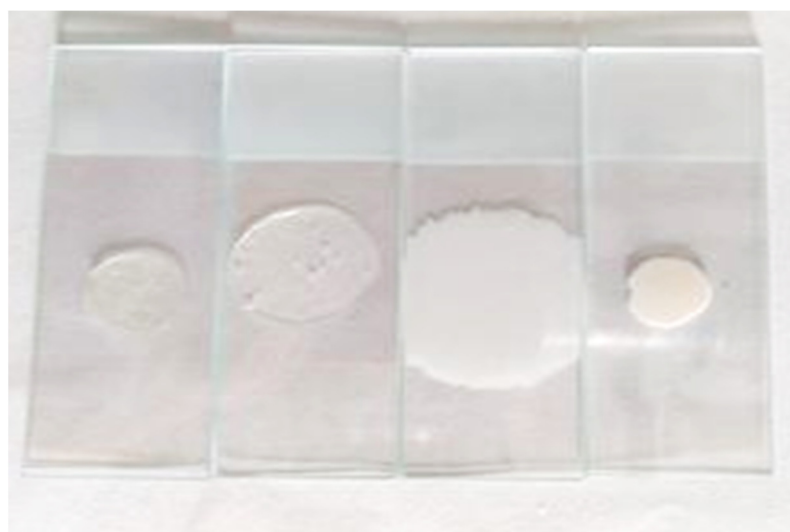
Figure 4. Tests of formulation spreading (0.07 g). From left to right: peel-off mask; water-soluble mask; cream; lip balm.
