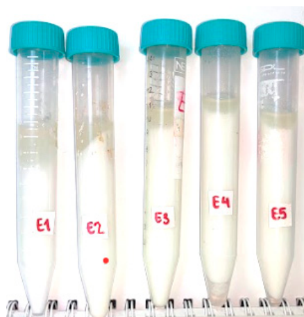
Figure 2. Facial cream subjected to centrifugal test after accelerated stability.
