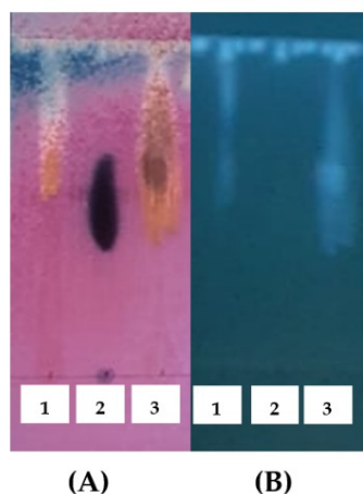
Figure 5. TLC analysis of glucose palm oleate synthesis from glucose and palm olein catalyzed by CPL. Lane 1; palm olein, lane 2; glucose, and lane 3; glucose palm oleate product. The TLC observation under (A) visible light and (B) UV light.
